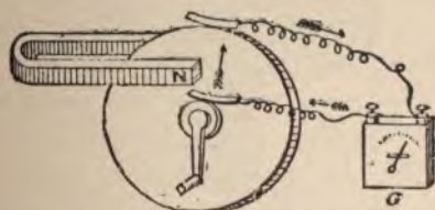
FIG. 64.—Faraday's electrical machine, the earliest dynamo constructed.
